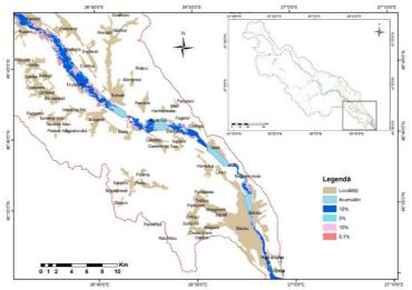
Fig. 7 Flooding maps with 10%, 5%, 1% and 0.1% assurance for the sector downstream Izvoru Muntelui Reservoir
